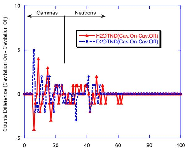
FIG. 3 (color online). Changes in counts from Neutron-Gamma Spectra for D<sub>2</sub>O and H<sub>2</sub>O with self-nucleation and BF<sub>3</sub> detector (counts for cavitation Off/On = 37/39 for D<sub>2</sub>O-UN; = 39/44 for H<sub>2</sub>O-UN).
