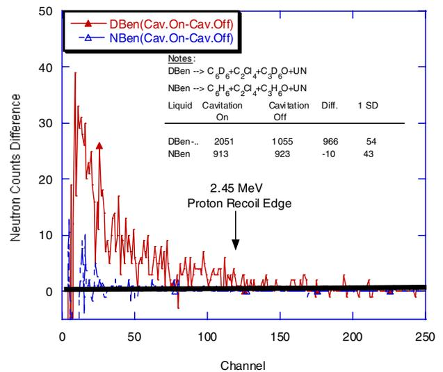
FIG. 4 (color online). Change in counts from pulse height spectra for C<sub>6</sub>D<sub>6</sub>-C<sub>2</sub>Cl<sub>4</sub>-C<sub>3</sub>D<sub>6</sub>O-UN and C<sub>6</sub>H<sub>6</sub>-C<sub>2</sub>Cl<sub>4</sub>-C<sub>3</sub>H<sub>6</sub>O-mixtures with self (alpha recoil nucleation) and LS detector (data taken over 300 seconds).
