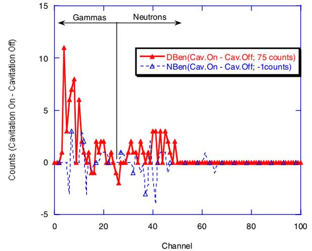
FIG. 2 (color online). Change in counts from Neutron-Gamma Spectra for  $C_6D_6$ - $C_2Cl_4$ - $C_3D_6O$ -UN and  $C_6H_6$ - $C_2Cl_4$ - $C_3H_6O$ -UN with self-nucleation and BF<sub>3</sub> detector (data collected over 3600 s; Cavitation off counts = 49 and 50 counts for deuterated and nondeuterated liquid tests, respectively).
